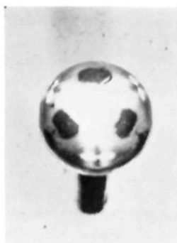
Fig. 5.—Action of a 7:1 mixture of hydrogen and oxygen on a copper single crystal at 400^{\circ} for sixteen hours. Normal to (111). Note strong reflection from area around (111) pole.
