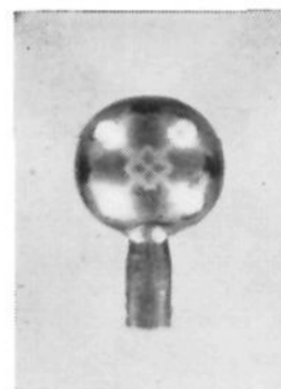
Fig. 4.—Action of a 7:1 mixture of hydrogen and oxygen on a copper single crystal at 400^{\circ} for sixteen hours. Normal to (100). Four bright lights were focused on (110) areas.
