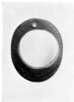
Fig. 2.—Typical appearance of a (100) slice exposed to a mixture of hydrogen and oxygen at 400^{\circ} for forty-eight hours.
