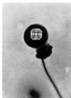
Fig. 3.—Action of a 7:1 mixture of hydrogen and oxygen on a nickel single crystal at 420^{\circ} for three days. Normal to (100).
