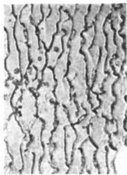
Fig. 10.—Action of a 7:1 mixture of hydrogen and oxygen on a copper single crystal at 400^{\circ} for sixteen hours: near (111), \times 600 .
